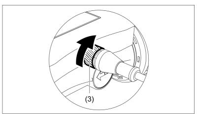
3. Connect the connecting cable to the device that is processing the signals and to the voltage supply. Route the cable so that it is protected against mechanical strain.
