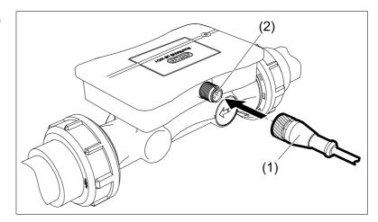
2. Screw the union nut (3) of the connecting cable onto the M12 plug connection on the device.
