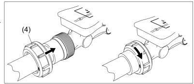
4. Switch on the plant, fill the pipe and check the tightness of the process connections under operating conditions.
